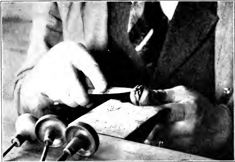
FIGURE 96. Filing the top of prongs
