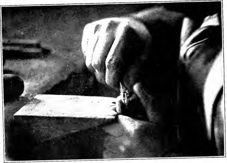
FIGURE 94. Setting the stone. First step
