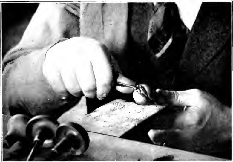
FIGURE 97. Bright cutting top and sides of prongs
