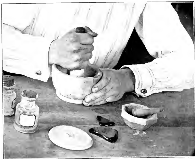
FIGURE 115. Grinding the Enamel
